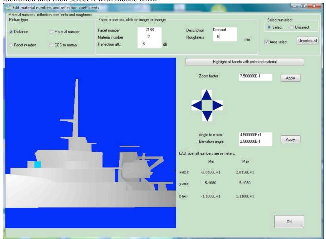
Then change Material number to 2 and Reflection att.: to -6 and Roughness to 5.
