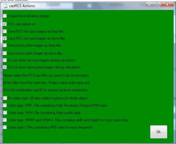
Select "RCS calculation on", "Save RCS hot spot images as micro files" and "Do not show mono pulse images during calculation.
