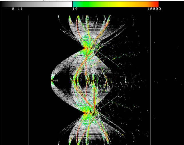
From both the first and second calculations with cadRCS without/with RAM we have the polar plots from movie, all plots are plotted as function of the azimuth angle and the data are the "Sum of range gates". The centre value of all plots is 20 dBsqm and outer value is 70 dBsqm. The plots are put together to one plot for each frequency. The lower RCS in the first quadrant of the plots are the calculations with RAM.
